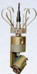
Well's Video camera with pan and rotate unit CCTV inspection for wells down to 400 meters in depth
